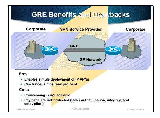
The figure shows two discontiguous networks, connected over a point-to-point logical link implemented over an IP network using a GRE IP tunnel. Such a tunnel is implemented on both border routers, and is visible in Cisco IOS as an interface.
