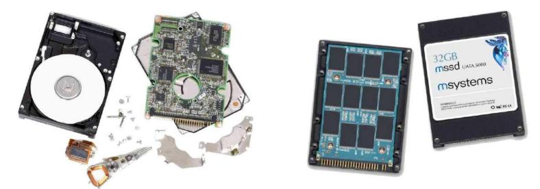
As you can see from the picture above, the main difference between a hard drive and a solid-state drive is that the solid-state drive is a lot more... well... solid! The lack of moving parts in the SSD is what gives it so many of its advantages, such as its speed and durability. There's a lot less that can go wrong when you don't have to worry about things wearing out or breaking.
