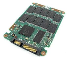
It's quite simple, really – MLC stands for *multi-level cell*, whereas SLC stands for *single-level cell*. This means that each *transistor* (or *cell*) in an MLC drive holds two bits of information, whereas in an SLC they only hold one.
